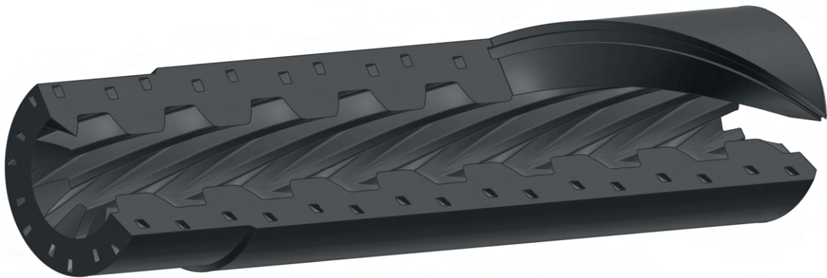
Figure 2.11: The fuel grain features a advanced twisted finocyl geometry. At the right hand side, the cut was implemented in the plane of one of the side ports to better visualize their swept geometry.
