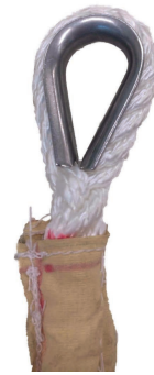
Figure 2.29: Thimble and rope protection.
