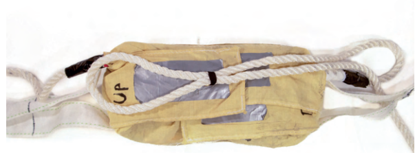
(b) Main bag closed. The main shock cord seals the bag in place.
