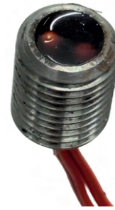
Figure 2.21: Chargecup with ignitors molded in PU.
