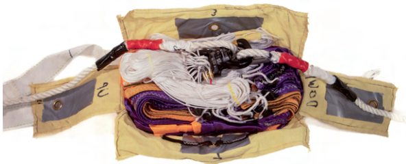
(a) Main bag opened. The folded main parachute is visible.
