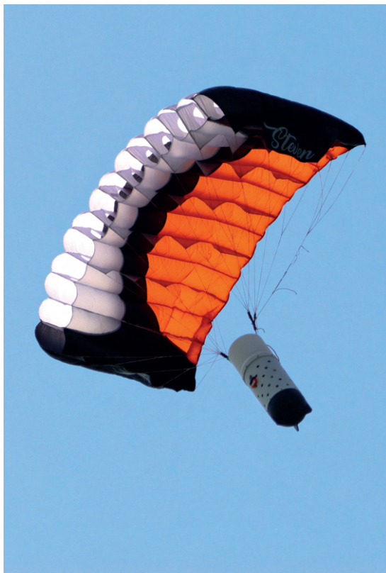
Figure 2.35: COTS parafoil during a test flight.
