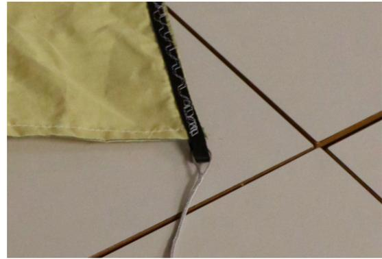
(b) Close up of a lash where the lines are connected.
