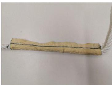
(a) Rope protection sewed onto the shock cords.
