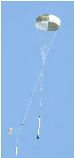
(a) Elliptical shape of the Main Parachute.
