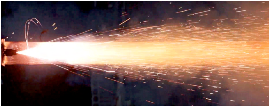
Figure 16: Dome-Sprayer during test firing. The length of the shot is approximately 130 cm.
