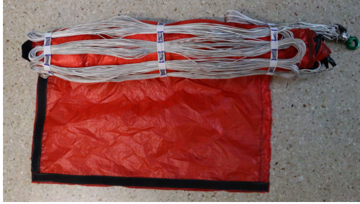
(a) Folded parachute is already packed and the lines are stored on the outside.
