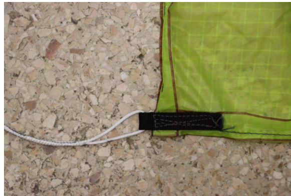
(c) Lashes where the lines are connected to the parachute.
