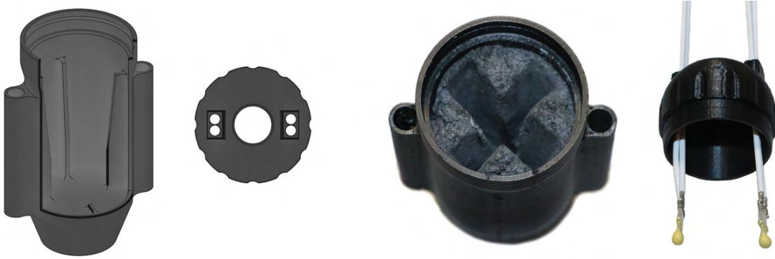
Figure 15: left: hull and lid of the Dome-Sprayer in Computer Aided Design (CAD), right: hull filled with pyrotechnic mixture and lid with inserted e-matches
