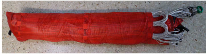
(b) Deployment bag sealed on the edges with velcro tape.
