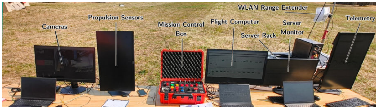
Figure 3.5: Mission control setup, antennas are not visible.
