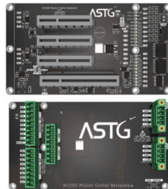
Figure 3.7: Mission control backplane.
