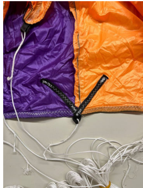
(b) V-lash on the skirt of the Main parachute.
