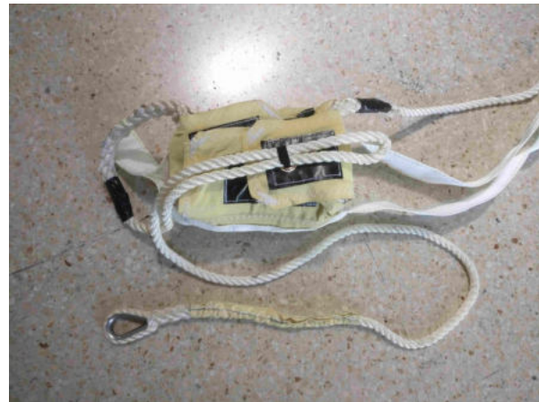
(b) The bag is held closed by the main shock cord.
