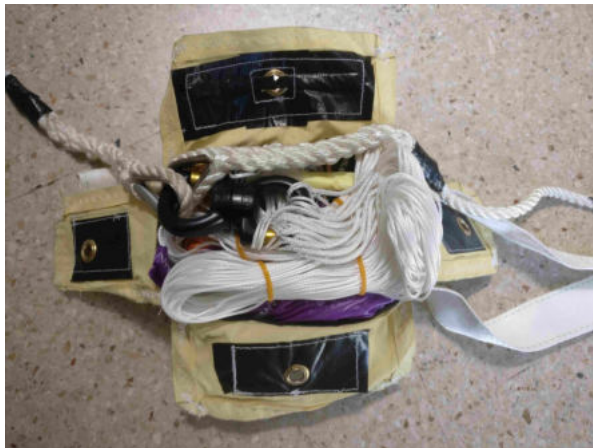
(a) The bag is open and has the main parachute with the lines and cords inside.
