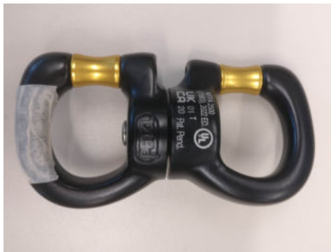
(a) The rotatable carabiner is used to decouple the spinning of parachute and rocket.
