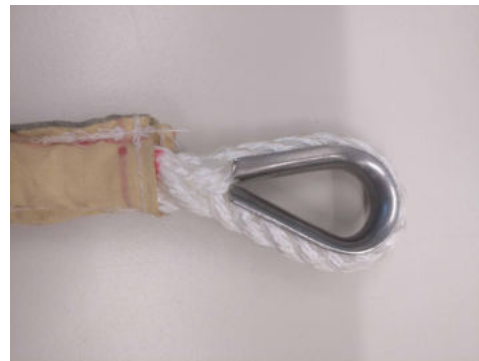
(b) The connection line is reinforced by a metal thimble and a Kevlar sleeve.
