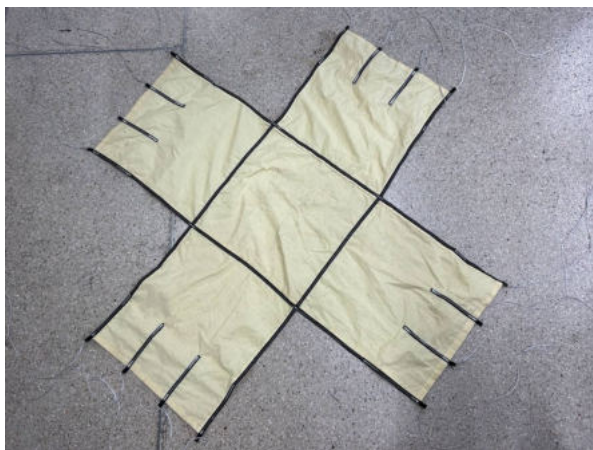
(a) Cross shape of the drogue parachute.
